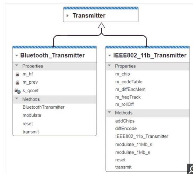
Example Transmitter classes in a wireless communications application.
